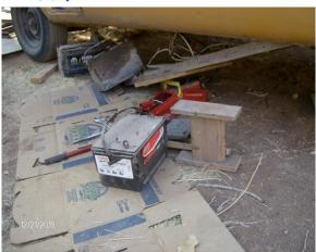
We use a home made battery pack and an inverter for power to run the lights, amplifier, copier, etc. A set of 4 twelve volt batteries. Three of them are bad.
